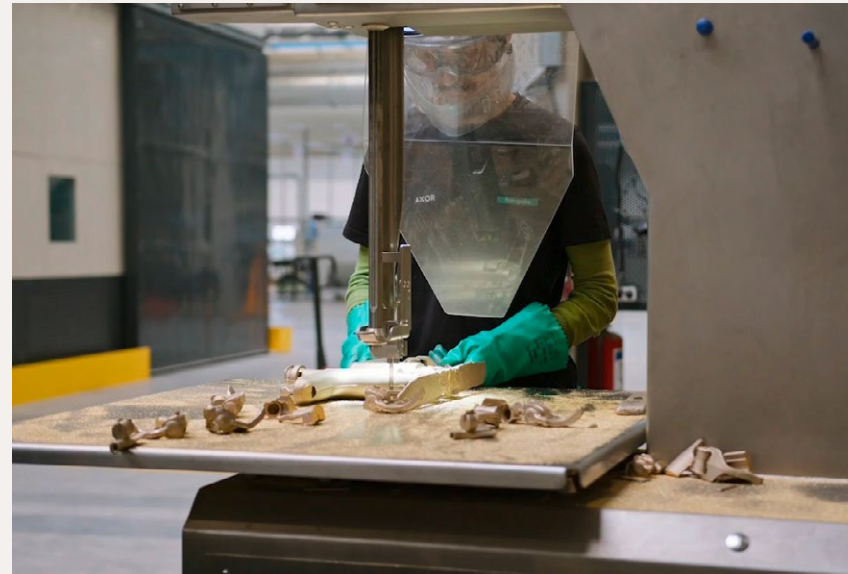
Workplace safety is a top priority: safety shields, gloves, and designated work areas ensure a safe process at the machine, as shown here during the deburring of a valve blank in the foundry.
