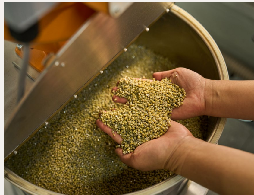
The recycled plastic pellets recovered from the processing plant are reintroduced into the cycle for the manufacture of new parts.
